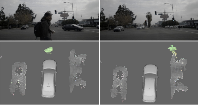
Fig. 12. A traffic scene showing a pedestrian crossing in front of the ego vehicle from left to right. Top: image snapshots from the corresponding traffic scene. Bottom: A part of estimated dynamic grid in the proximity of the ego-vehicle (top-view). The dynamic grid result shows a crossing pedestrian (green arrows). Additionally, the estimated grid includes the projection of two adjacent cars represented by white dots (not visible in the top camera images). The ego vehicle, as well as the other two left and right cars are stopped at the traffic light. It can be seen that as soon as the crossing pedestrian passes closer to the static obstacle (in front of the right vehicle), some of the pedestrian velocity vectors are temporarily biased by the wrong associated measurements belonging to stationary vehicle.
