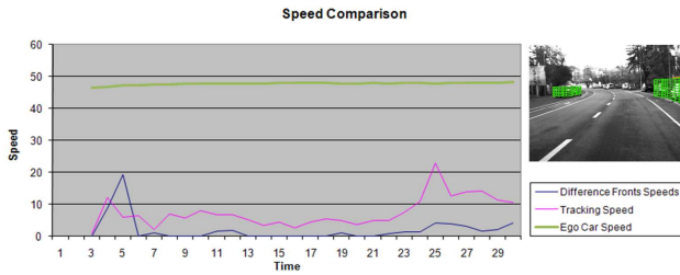
Figure 7. Speed Estimation for a stationary lateral vehicle (green color). The results are estimated with particle based tracking of difference fronts (blue color), Kalman filter tracking (magenta color). The ego car speed is colored with green.
