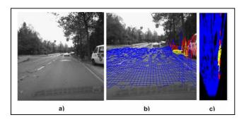
Figure 2. The Occupancy Grid (c) is computed from the Elevation Map (b) of a scene (a). The occupancy grid cells are roughly classified (blue – road, yellow – traffic isle, red – obstacles)
