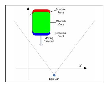
Figure 3. In a Difference Map, we have two types of difference fronts that characterize moving objects between two frames: in the direction front (with blue) the occupancy grid cells are present in the current frame but are empty in the previous frame, the shadow front flags the cells that are empty in the current frame but are filled in the previous one
