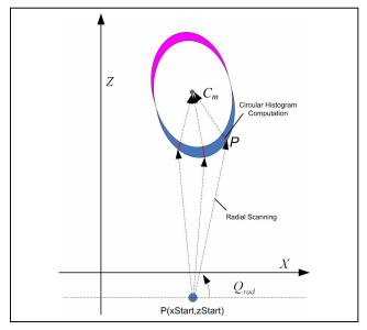
Figure 4. Accumulating the difference points that fall into the circular histogram associated to an object.
