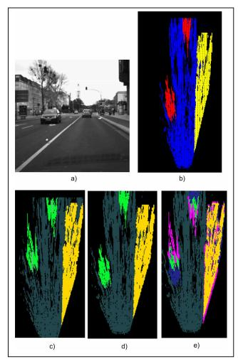
Figure 6. Temporal Difference. The Occupancy Grid (b) is computed from scene (a). The temporal difference (e) uses the previous occupancy grid (c) corrected with the ego motion, and the current occupancy grid (d). The Temporal Difference Maps Cells are classified in shadow cells (magenta), direction cells (blue), traffic isles core cells (yellow), and obstacles core cells (light green)
