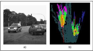
Figure 5. Difference Map (b) of the scene (a). Circular histograms (colored with orange) are computed. The mean directions (colored with red) are associated to the corresponding moving obstacles.
