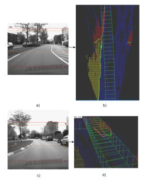
Figure 6. Collision Detection: a) Left camera image. b) Collision detection - Top View. c) Left image. d) Collision detection - Free Look.
