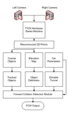
Figure 1. System Architecture
