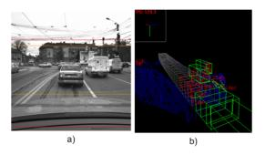
Figure 7. Collision Detection: a) Left camera image. b) The generated tunnel does not include any delimiter
