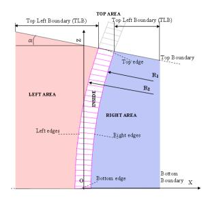
Figure 5. Drivable Tunnel model projected on the xOz plane (top view)
