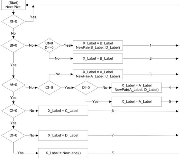
Fig. 5.2 Block diagram of the labeling algorithm
