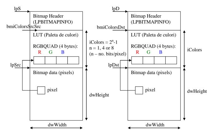
**Fig. 1.7**. Structure of a bitmap (with LUT – 1, 4 or 8 bits / pixel) in the memory (source image and destination image).
